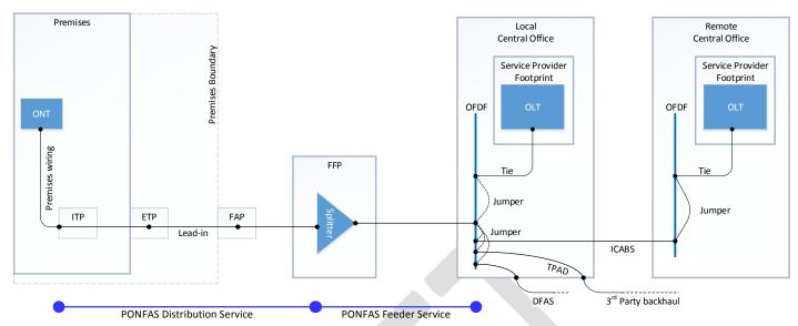
This is a generic diagram showing the standard configuration and service demarcation points. It is not intended to represent every situation or detailed physical architecture. The following points should be noted:
