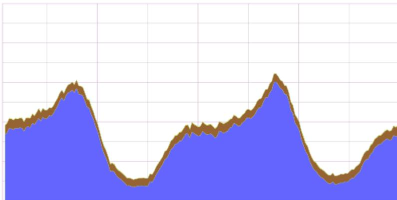
It should be noted that High traffic class demand is relatively smooth throughout the day, while Low traffic class demand increases until the (current) peak hour of around 9pm. Therefore investment in broadband capacity in New Zealand is driven by peak hour, Low traffic class.
