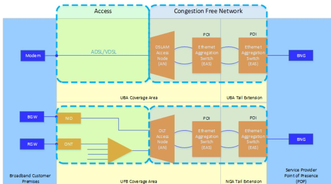
The access lines are excluded due to the low levels of contention of these portions of the network, as described below.
